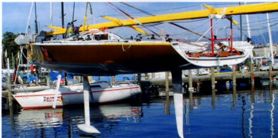
Light and flat, and with twin high-aspect daggerboards (port foil partly extended, above ), the Psaros 40 has proved a successful lake racer as well as an unusually reliable one!
